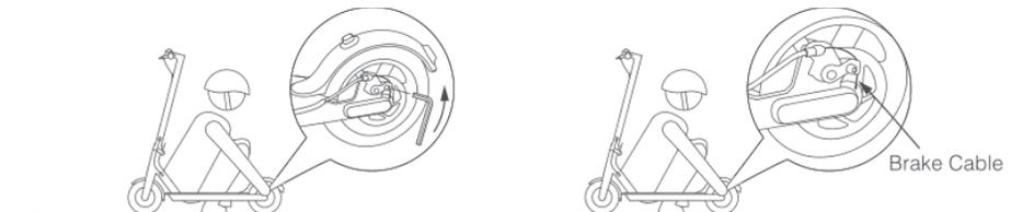
If the brake is too tight, use the M4 hexagon wrench to loosen the screws on the caliper, and slightly send back the brake cable to shorten the exposed length, then tighten the screws. If the brake is too loose, loosen the screws, and slightly pull out the brake cable to lengthen the exposed length, then tighten the screws.
